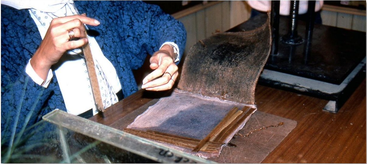
Modern papyrus maker, arranging overlapping vertical and horizontal strips of papyrus. To the right is a press for pressing the layers together.
